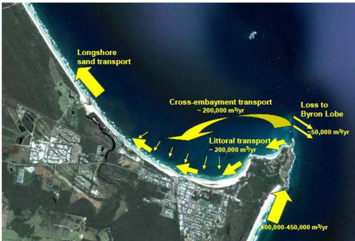
Figure 3.3 Conceptual sand transport (BMT WBM, 2013)
