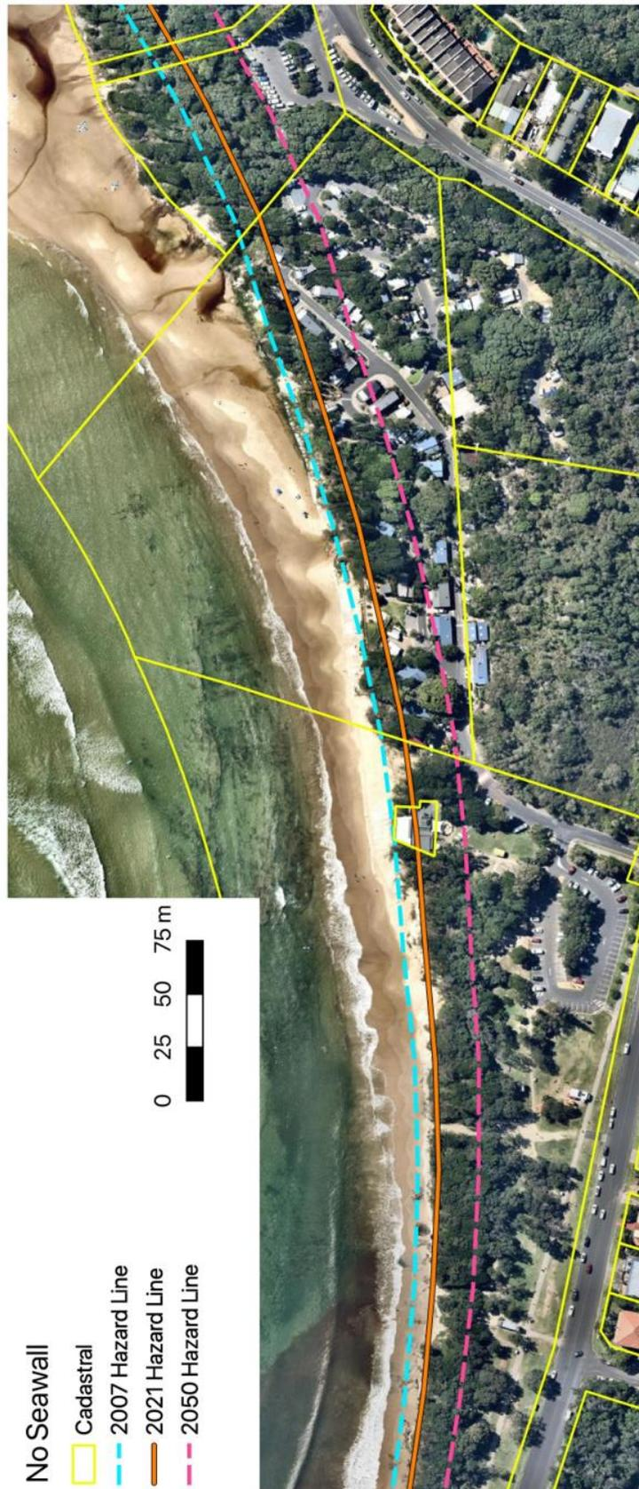
**Figure 7.9 Erosion-recession hazard lines – close up**
