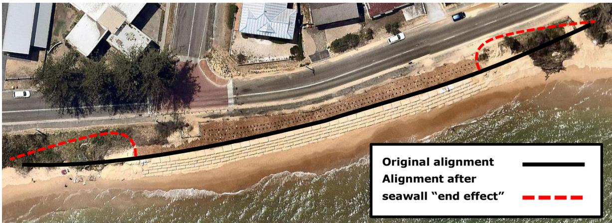
**Figure 3: Potential seawall erosion "end effect"**
